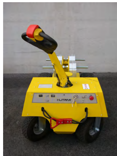
The handle directs two steering wheels and the drive controller operates from the drivers thumb.
