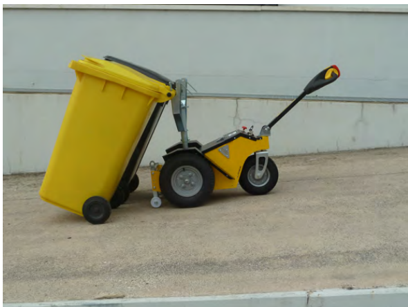
TT600 complete with optional Front Hook and Anti Dumping Wheels & 240 litre bin attachment and
